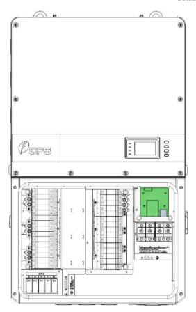
The CPS Flex Gateway is a new communications and controls solution for the CPS 36, 50, 60, 100 and 125kW inverters. The gateway is a Modbus master data logger and communications device. This flexible solution enables three parallel outbound communication options: (1) local pass-through Modbus RS485 data to 3rd party solutions, (2) Ethernet based communications for CPS service operations, and (3) a programmable Ethernet based connection to a location chosen by the customer.
